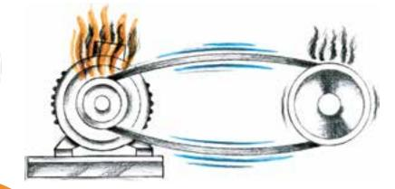
Prevents from slack accruement, avoids heat generating slippage of the belts and averts from premature belt failure!
