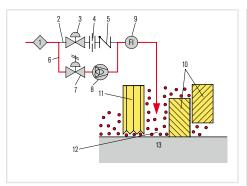
Operating and installation diagram for a RoTechBooster
