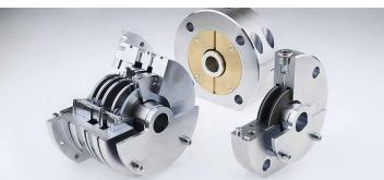
Carbon floating ring seals are supplied as maintenance-free compact labyrinth cartridge seals with low leakage. The floating self-adjusting sealing rings provide radial sealing on the shaft with a very small gap. The seal requires no additional lubrication, and it is designed for dry running. Besides pure gas, carbon floating ring seals are also suitable for Atex applications, toxic media, media containing solids, flue gas, dust, powder, vapor, liquid mist, oil mist and penetrating oil.
