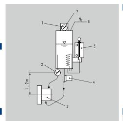
Operating and installation diagram for a TS1000 system.
