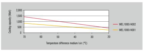
Cooling capacity: Values based on moved air min. 0.7 m/s and barrier fluid water.
