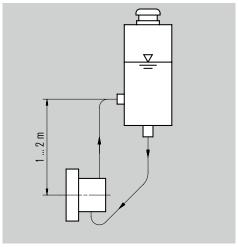
Install the quench fluid tank approx. 1 ... 2 m (3.3 ... 6.6 ft) above the mechanical seal. Install connection pipes To mechanical seal with low flow resistance. Pipes must vent automatically in the direction of the tank. It is imperative that air pockets are prevented. The minimum filling level must always be above the connection socket at the side (in the case of the thermosiphon principle). Quench fluid systems can be operated in two different modes.
