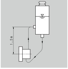
Install the quench fluid tank approx. 1 ... 2 m (3.3 ... 6.6 ft) above the mechanical seal. Install connection pipes To mechanical seal with low flow resistance. Pipes must vent automatically in the direction of the tank. It is imperative that air pockets are prevented. The minimum filling level must always be above the connection socket at the side (in the case of the thermosiphon principle). Quench fluid systems can be operated in two different modes.
