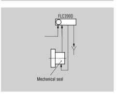
P&ID for FLC200 for single mechanical seals, FLC200Q for mechanical seals with quench and FLC200D for dual mechanical seals.
