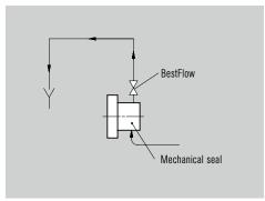
Installation diagram for a BestFlow valve.
