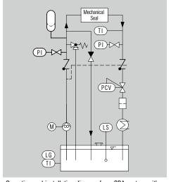
Operating and installation diagram for a SPA system with a  $\mathbf{DHE}$
