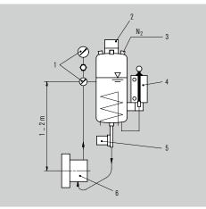
Operating and installation diagram for a TS5000 system.
