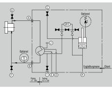
Operating and installation diagram for SPO (Plan 53C)
