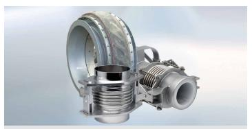
Expansion joints are vital components in most industrial plants. They are installed as flexible connections in pipe and duct systems to take up or compensate for thermal expansion, vibration and misalignments. Advancements in processing and generating technologies are being combined with high demands for efficiency. This, along with a clear orientation towards environmental protection, puts high demands on expansion joint designs.
