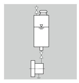
Install the quench fluid tank above the mechanical seal.
