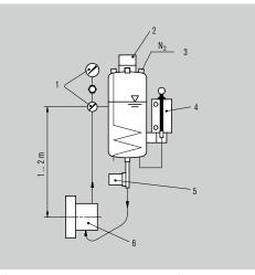
Operating and installation diagram for a TS4000 system.
