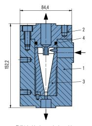
ZY61 in block-type design with integrated flange
