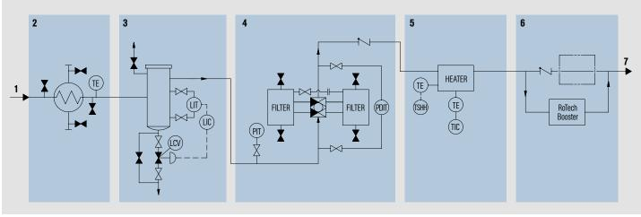
Example of a gas conditioning system (skid).
