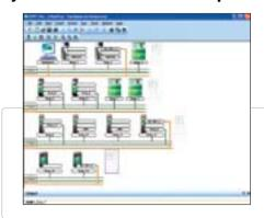
SyPTPro is a full featured automation development environment that can be used for developing tailored solutions for single or multiple drive applications. The programming environment fully supports three industry standard languages: Function Block, Ladder and Structured Text. Motion control is configured using the new PLCopen motion language, supporting multiple axes.
