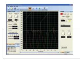
CTScope is a full featured software oscilloscope for viewing and analysing changing values within the drive. The time base can be set to give high speed capture for tuning or for longer term trends. The user interface is based on a traditional oscilloscope, making it familiar and friendly to all engineers across the globe.
