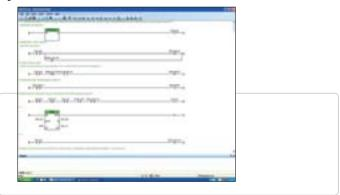
Mentor MP has an inbuilt programmable controller. It is configured using SyPTLite, an easy-to-use ladder logic program editor, suitable for replacing relay logic or a micro PLC for simple drive control applications.
